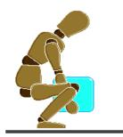
Don't flex the back any further while lifting. This can happen if the legs begin to straighten before starting to raise the load.
