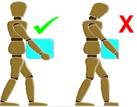
Put down, then adjust. If precise positioning of the load is necessary, put it down first, then slide it into the desired position.
